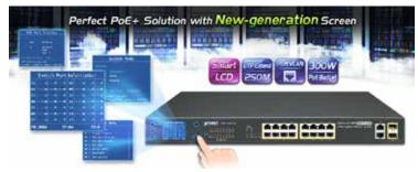
The FGSW-2622VHP is equipped with **24 10/100BASE-TX** ports taking up 30 watts of PoE+ power each and **2 Gigabit TP and 2 Gigabit SFP** interfaces with inner power system. With a total PoE+ power budget of **300 watts** and nonblocking data switching performance, the FGSW-2622VHP can fulfill the demand of sufficient PoE power for HD IP surveillance. It offers a desktop-sized, reliable and visible power solution for small businesses and system integrators deploying Power over Ethernet networks.
